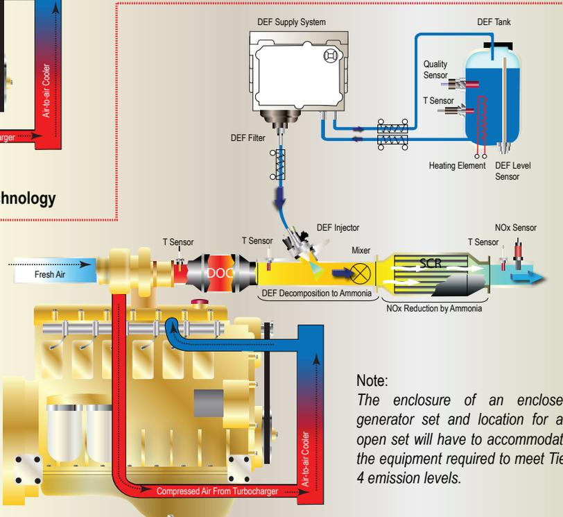
**Selective Catalytic Reduction and a Diesel Oxidation Catalyst**
