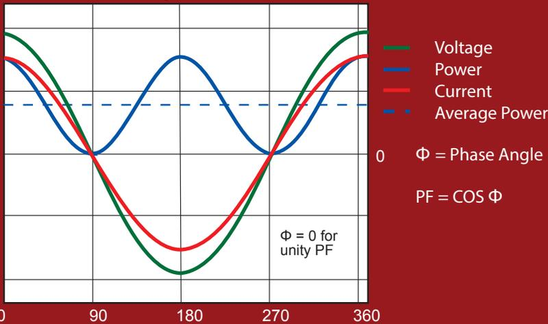
Purely resistive load connected with volts and amps in step for an unity (1) power factor when all the source energy is transferred and available to the load. Good power factors are normally greater than 0.9 to 0.95.
