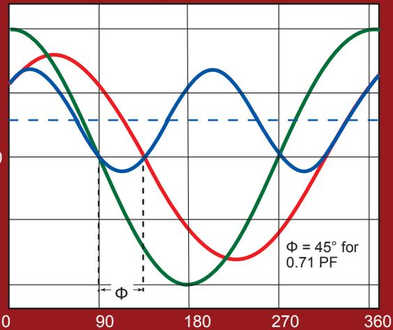
Inductive load connected with current waveform lagging volts. Below unity PF only a percentage of the power is available at the load. i.e 0.8 PF has real power 80% of apparent power. Reactive loads have a percentage of power returned to the source.
